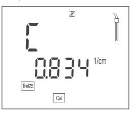
5 Switch to the measuring mode with **<ENTER>**. The determined cell constant is used.
