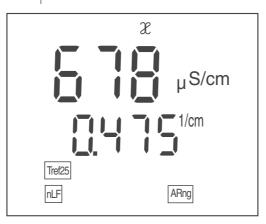
4 Confirm the selection with **<ENTER>**. The meter switches to the measured value display.
